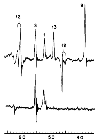
Figure 1. 1 H NMR spectrum (60 MHz) of diazoacetone (1; 0.1 M) in CHCl 3 (bottom) and CIDNP spectrum observed during the photosensitized decomposition (benzophenone, 0.1 M) of 1 in CHCl 3 (top). S denotes the high-field 13 C satellite of CHCl 3 .
